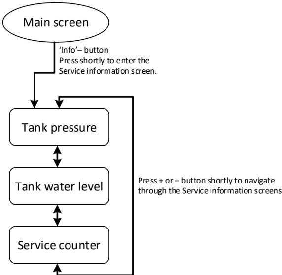
Figure 51. Structure of the service information screens for the VERNIT Basic
