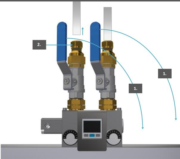
Figure 35. Loosen HP-vessel pipe
