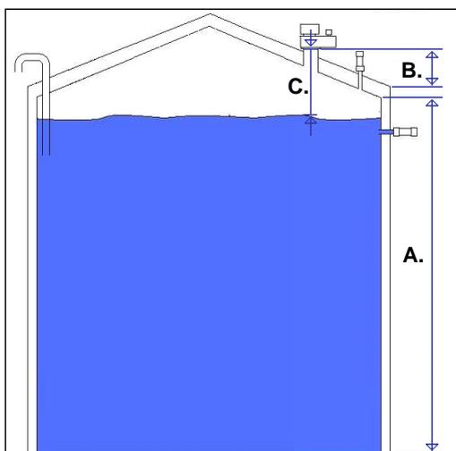
Figure 32. Measuring the water level
