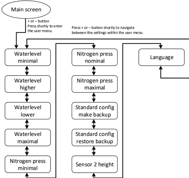
Figure 50. Structure of user menu of Vernit Basic system
