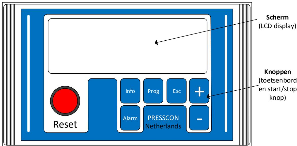
Figure 49. Schematic view of Press-display
