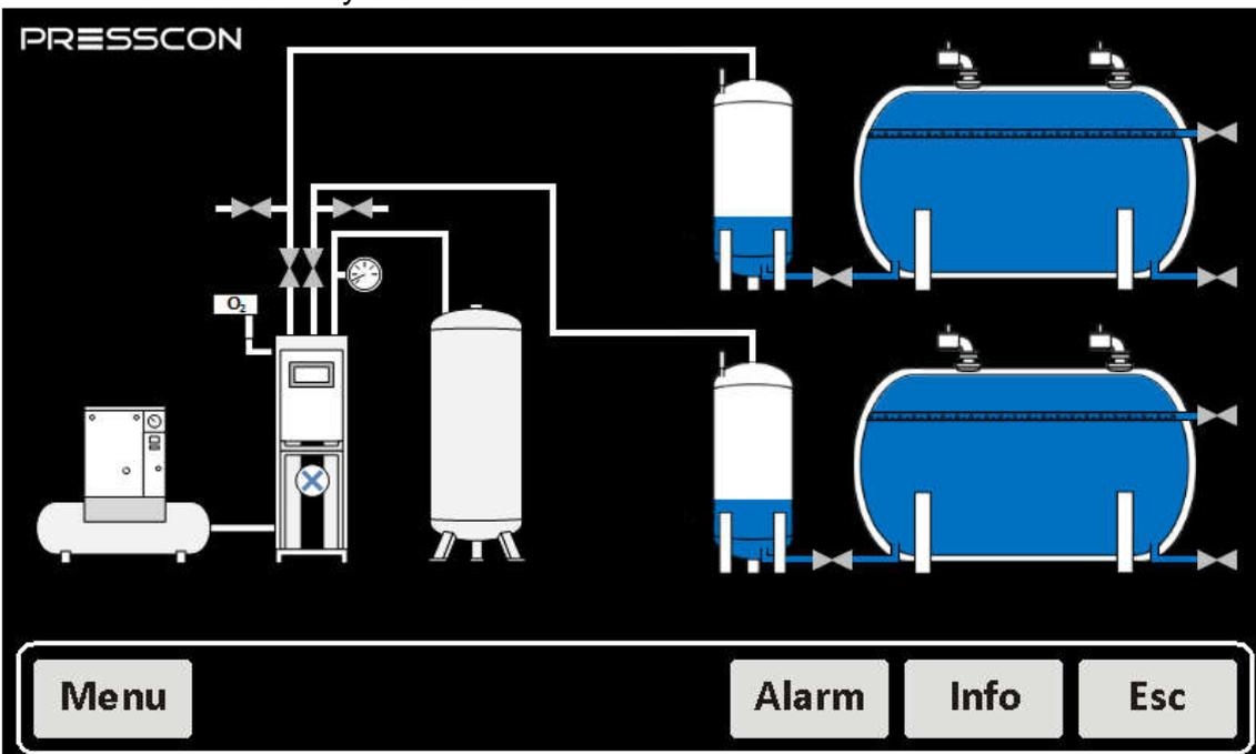
Figure 47. HORNIT 2.0 – 30.0 N2(i) DUO system overview (Only when the HORNIT is installed)
