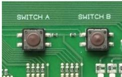
Figure 45. Switch A and B on the PCB of the PRESS-control
