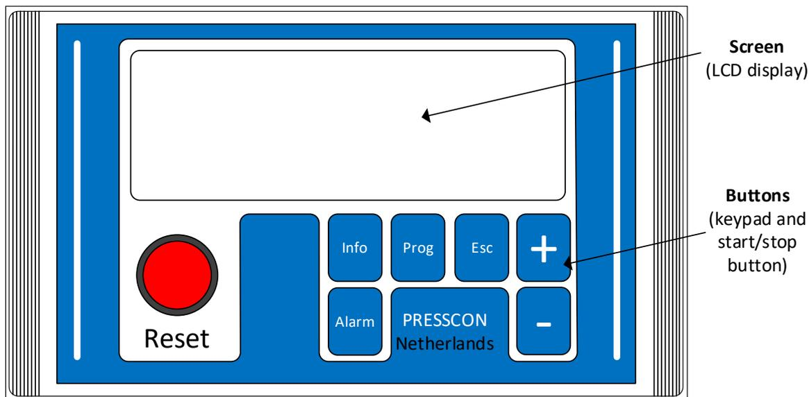
Figure 9. Schematic view of Press-display
