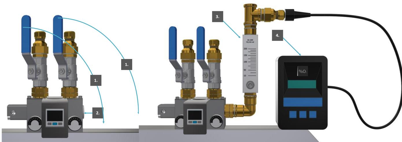
Figure 39. Measuring flow and purity
