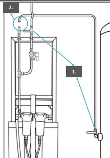
Figure 36. Loosen HP-vessel pipe, old type of system
