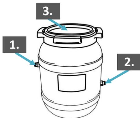
Figure 15. Oil Water separator
