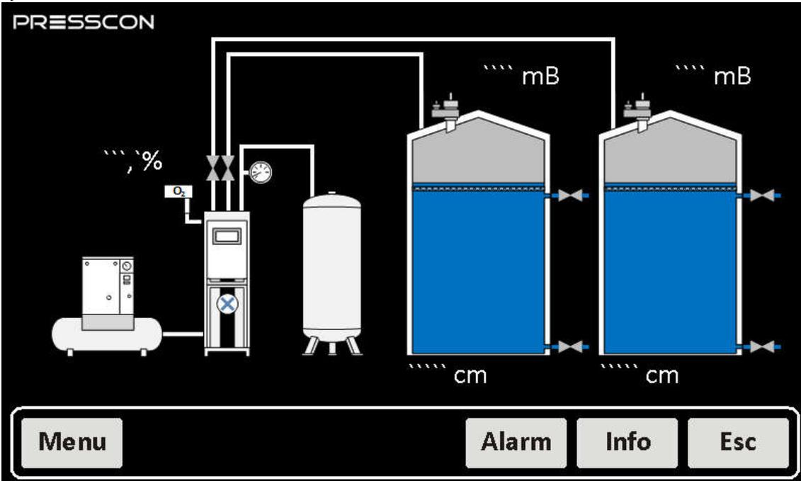
Figure 46. VERNIT 2.0 – 30.0 N2(i) DUO system overview (Only when the VERNIT is installed)
