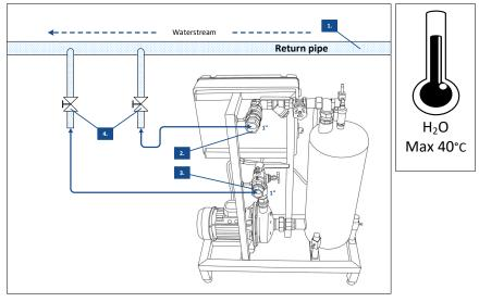
Figure 4. Connection to return pipe
