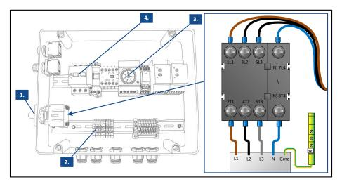
Figure 5. ExitOxy switch panel
